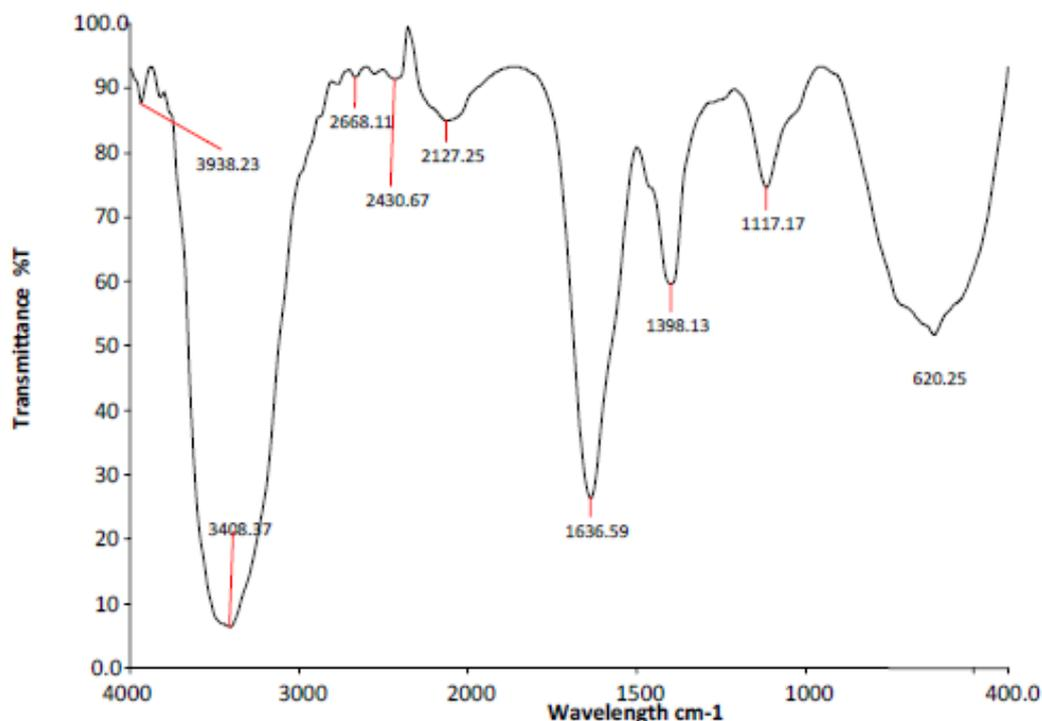
Figure 2a. The FTIR spectrum of a control dye FTIR Results
