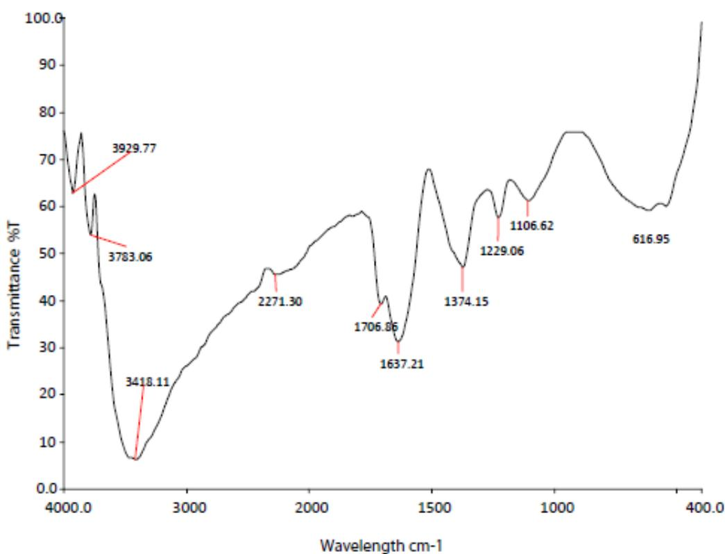
Figure 2b. The FTIR spectrum of extracted metabolites (24 hours)
