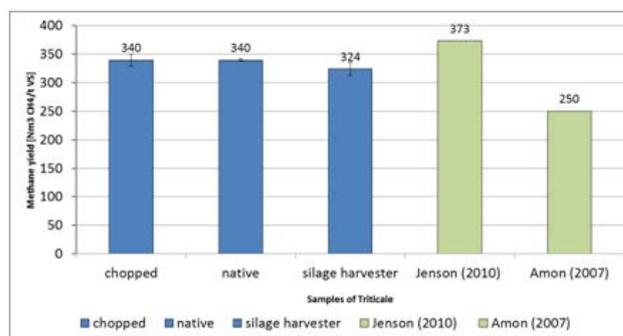
**Figure 10.** Biogas production over 47 days of incubation at 37°C
