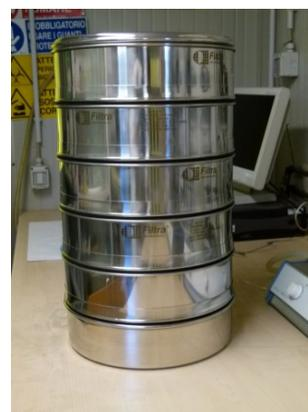
**Figure 4.** Series of sieves used for particle size analysis
