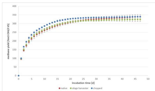
**Figure 9.** Biogas production over 47 days of incubation at 37°C
