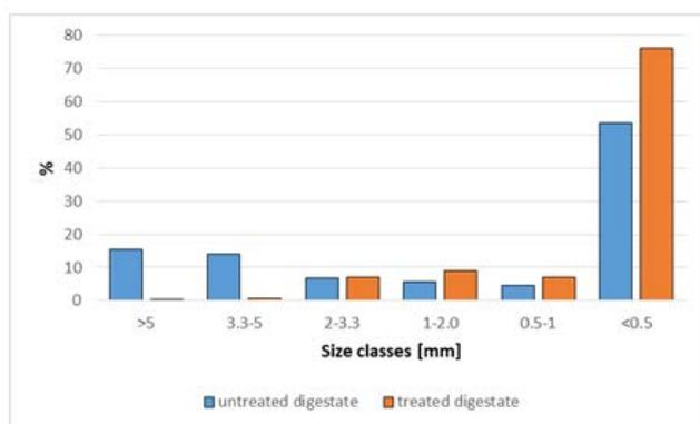
**Figure 8.** Percentage size distribution of the particles of an untreated digestate and treated digestate sample [20]
