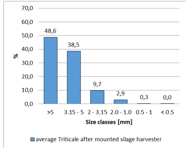
Figure 6. Granulometric distribution of triticale after treatment with mounted silage harvester
