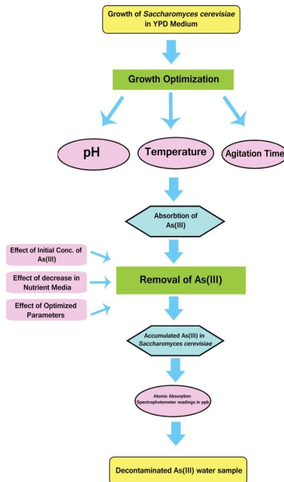
Figure 1. General schematic representation of biosorption process
