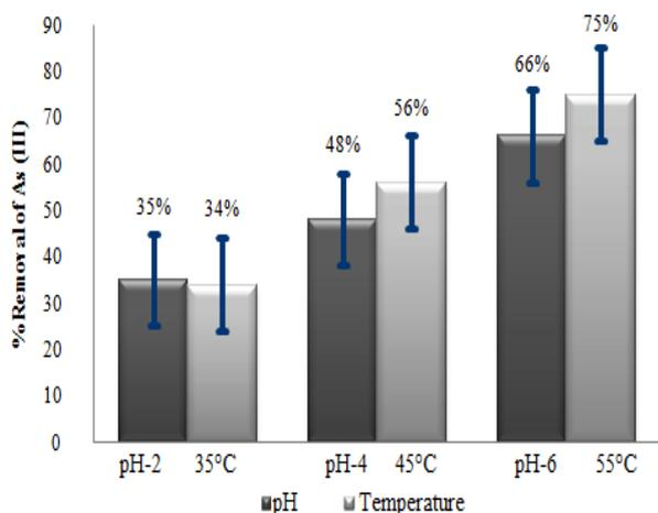
**Figure 5.** Percentage removal of As (III) with respect to pH and percentage removal of As (III) with respect to temperature
