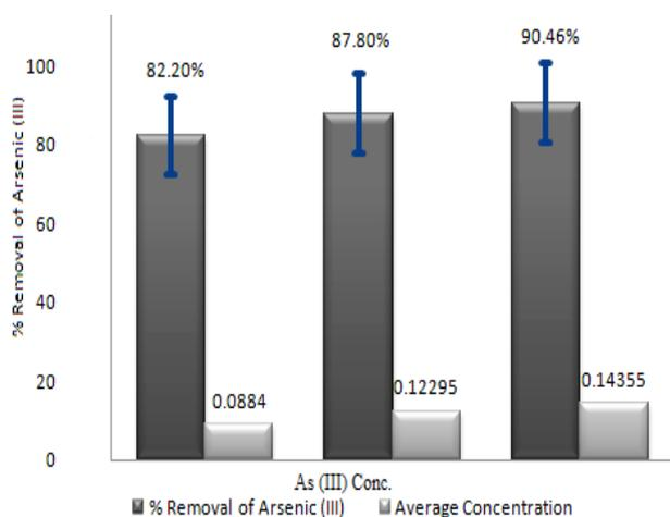
**Figure 3.** Percentage removal of As (III) with respect to varying initial concentration and the average concentration
