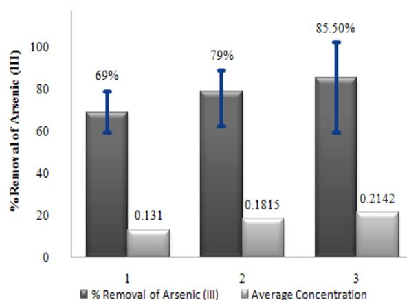
**Figure 2.** Percentage removal of As (III) with respect to decrease in nutrient media, increase in initial As (III) concentration and average conc (In graph: 1-0.2 mg/l; 2-0.3 mg/l; 3-0.4 mg/l)
