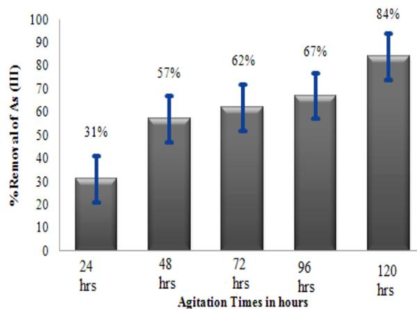
**Figure 4.** Percentage removal of As (III) with respect to agitation time
