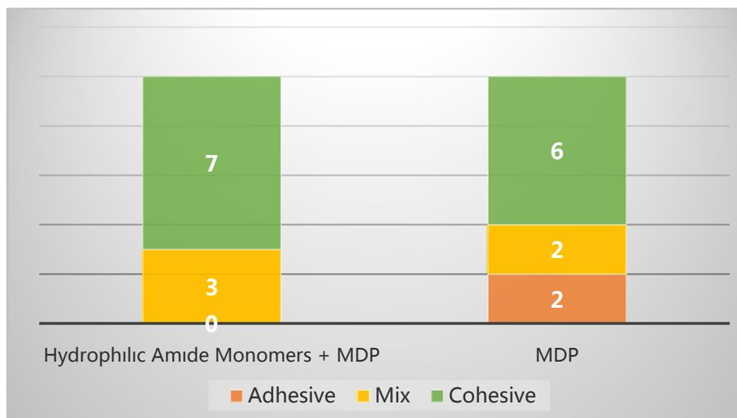
**Figure 1. Fracture patterns**
