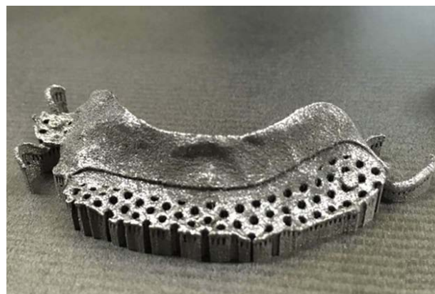
Figure 6. Titanium framework after removing from the SLM machine
