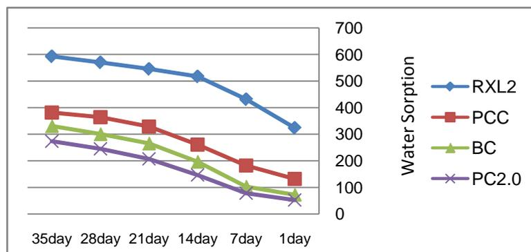
**Figure 3.** Water sorption ( $\mu\text{g}/\text{mm}^3$ ) of each cement at different time intervals
