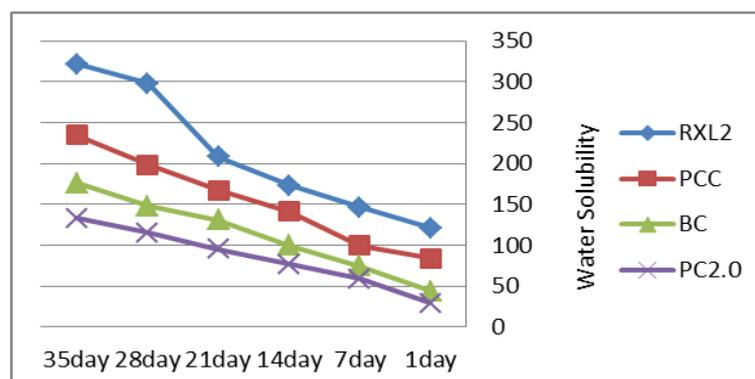
**Figure 4.** Water solubility ( $\mu\text{g}/\text{mm}^3$ ) of each cement at different time intervals
