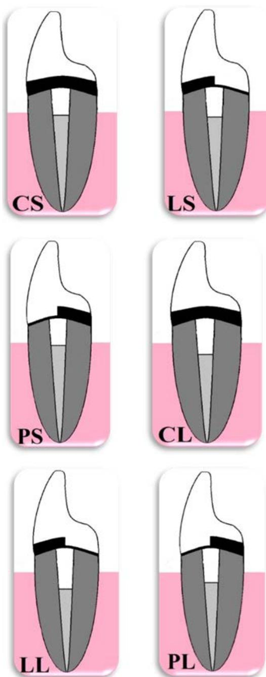
Figure 1. Different endocrown designs with different residual coronal tooth structures. CS, 2mm circumferential with 2 mm radicular depth, LS, residual labial wall with 2 mm radicular depth, PS, residual palatal wall with 2 mm radicular depth, CL, 2mm circumferential with 4 mm radicular depth, LL, residual labial wall with 4 mm radicular depth, and PL, residual palatal wall with 4 mm radicular depth
