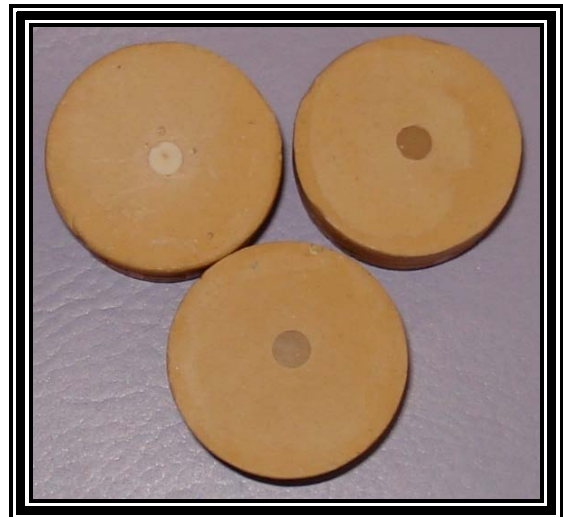
Figure 2. The specimens of the Glass-ionomer based materials mounted in stone blocks for microhardness assessment
