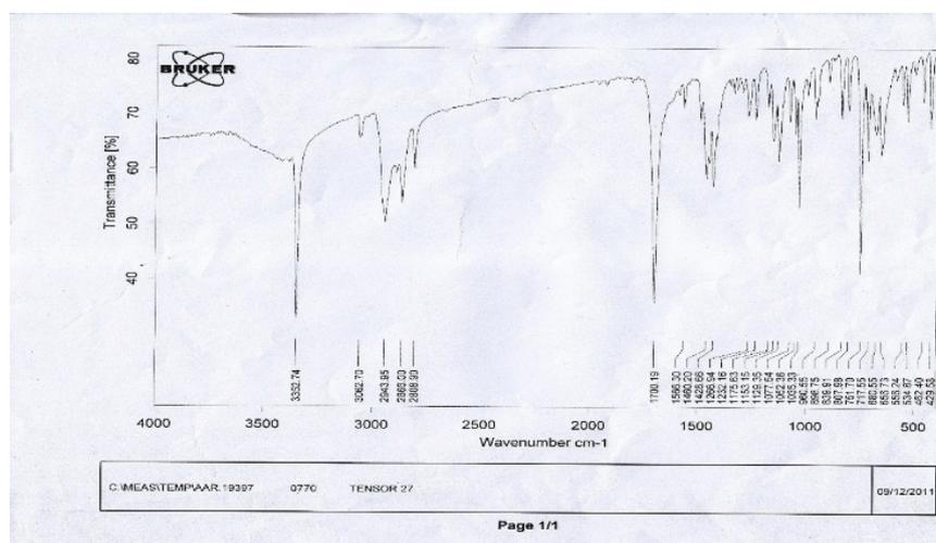
Figure 3. Pure ketamine extract measurement by FTIR (Infra-red) spectroscopy
