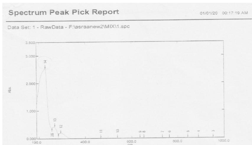
Figure 4. Pure ketamine extract measurement by UV (Ultra-Violet) Spectroscopy
