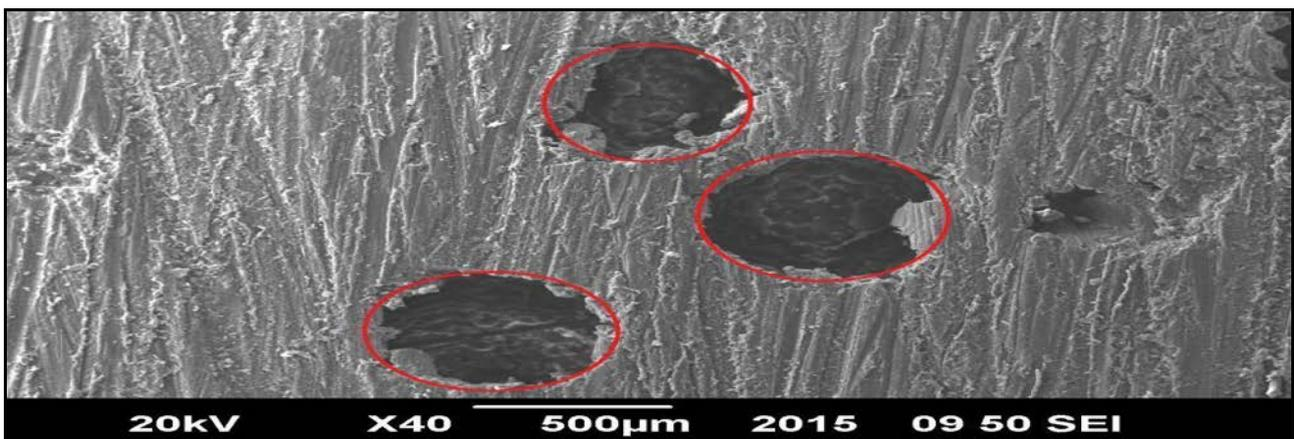
Figure 3. Porosity perimeter outlined for measurement
