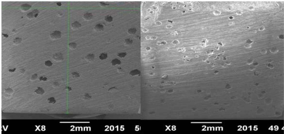
Figure 7. SEM images of specimen cured according to Cycle 2A and 2B
