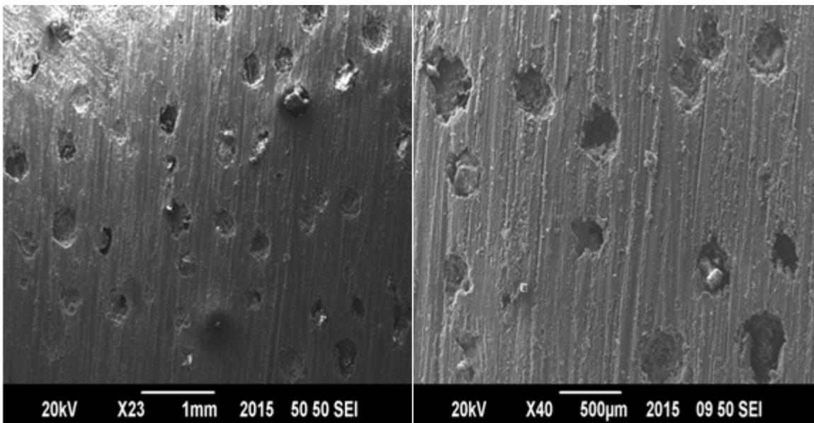
Figure 6. SEM images of specimen cured according to Cycle 1A and 1B
