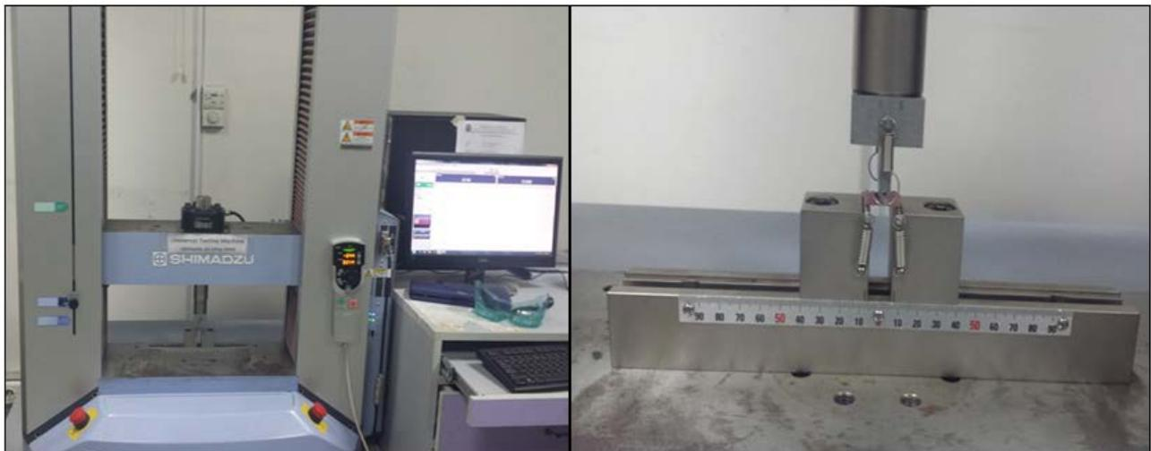
Figure 2. Testing for flexural strength of acrylic specimens
