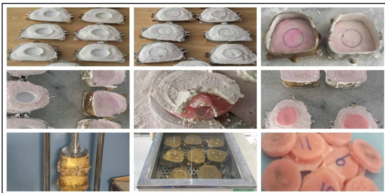
**Figure 1.** Preparation of the acrylic specimen
