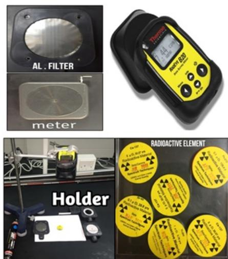
**Figure 1.** The Aluminum filter, holder with adjustable screwed arm, radioactive sources and radiation survey detector (RedEye B20-version – 2,19V E.2.05 / 2012-09-07)
