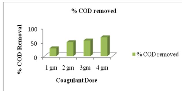
Figure 9. Effect of (Alum) coagulant dose on the COD removal efficiency
