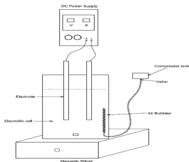
**Figure 1. Electro coagulation Treatment**
