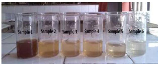
Figure 7. Colour Removal Efficiency by using Electro coagulation (EC)
