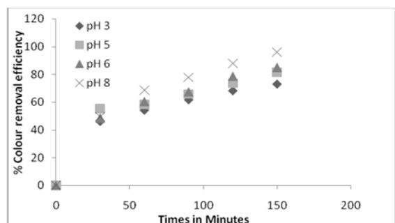
Figure 6. Effect of pH on efficiency of Colour removal for Al-Al Electrodes
