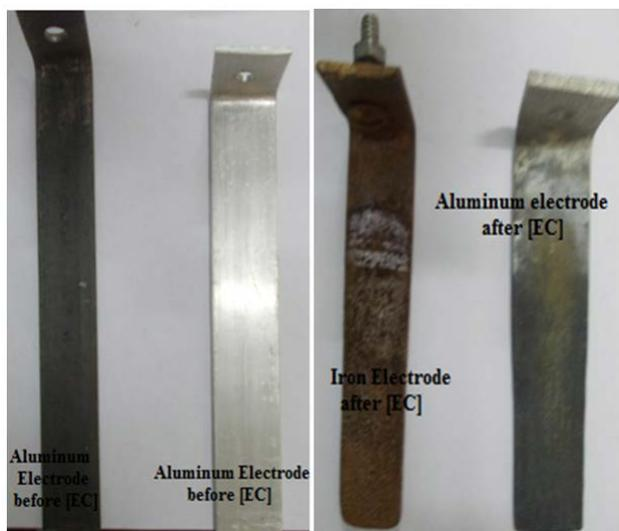
Figure 8. Electrodes before and after [EC]
