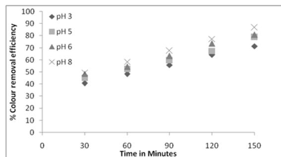
Figure 5. Effect of pH on efficiency of Colour removal for Fe-Fe Electrodes
