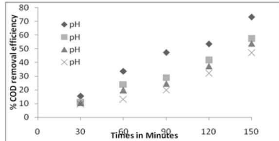
Figure 4. Effect of pH on efficiency of COD removal for Fe-Fe Electrodes
