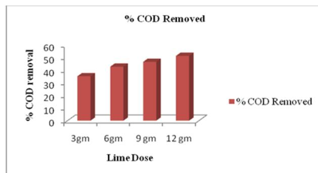
Figure 10. Effect of (Lime) coagulant dose on the COD removal Efficiency
