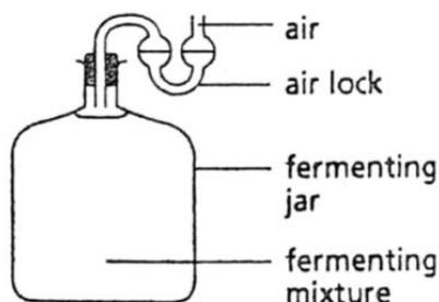
**Figure 7.** The apparatus used for fermentation
