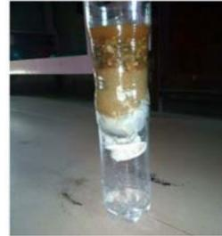
**Figure 5.** Pour well water into the filter system
