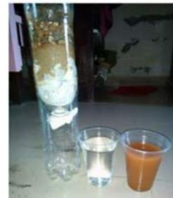
**Figure 6.** Water obtained after filtration (cup in the middle)
