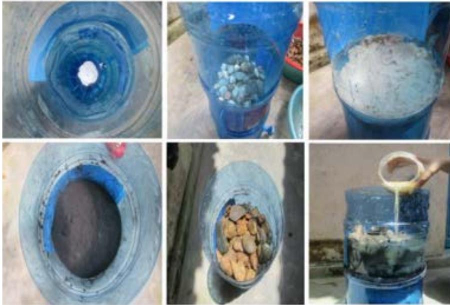
Figure 9. Sort the filter materials and carry out filtering dirty water
