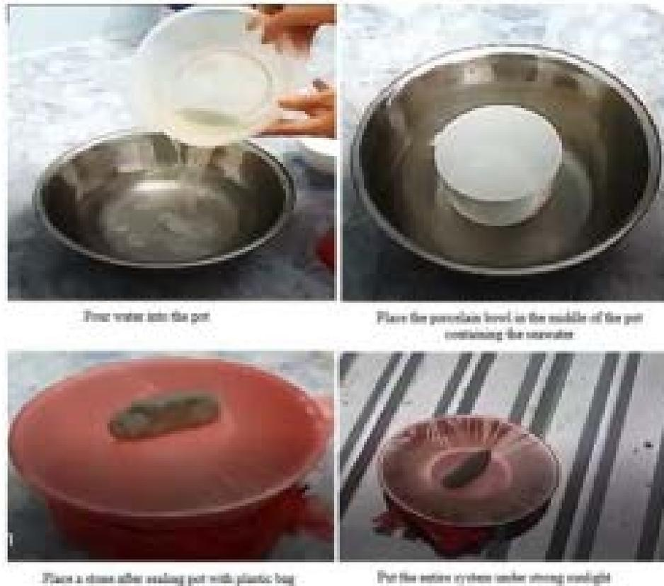
Figure 12. Carry out filtering water
