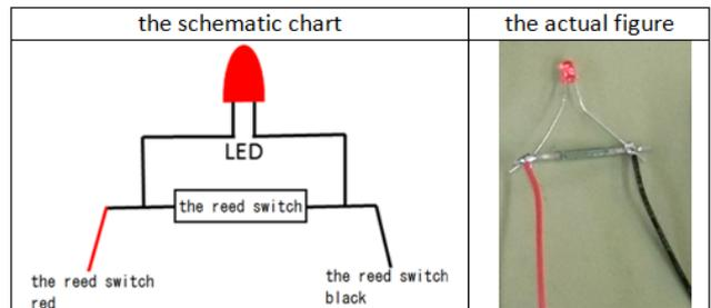
Figure 2. The reed switch and LED
