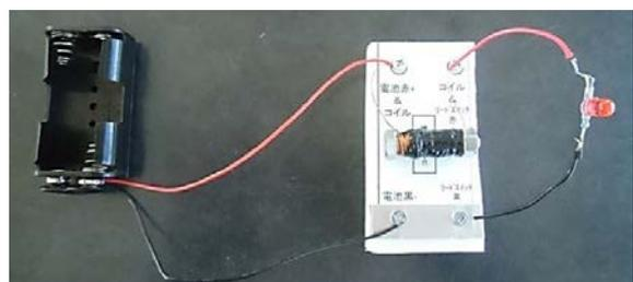
Figure 4. Completed model of the magnetic top
