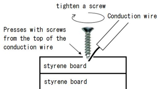
Figure 3. Connection of conduction wire by screws
