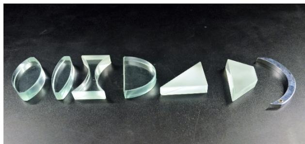
Components: Converging lens, Diverging lens, Semi-cylindrical lens, rectangular prism, trapezoidal prism, concave mirror.
