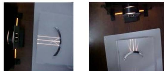
Experimental setup to get focal distance. the mirror concave and convex
