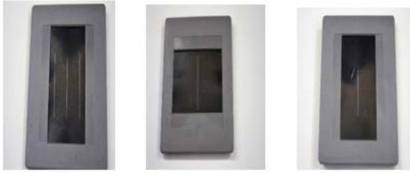
Three slots diaphragms. Single slots diaphragms, Object slots diaphragms.
