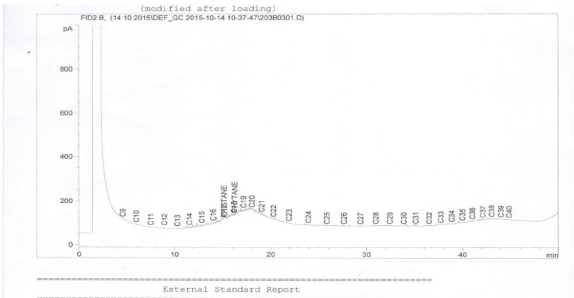
Figure 3. TPH (n-alkanes) chromatogram of oil from Bodo soil sample
