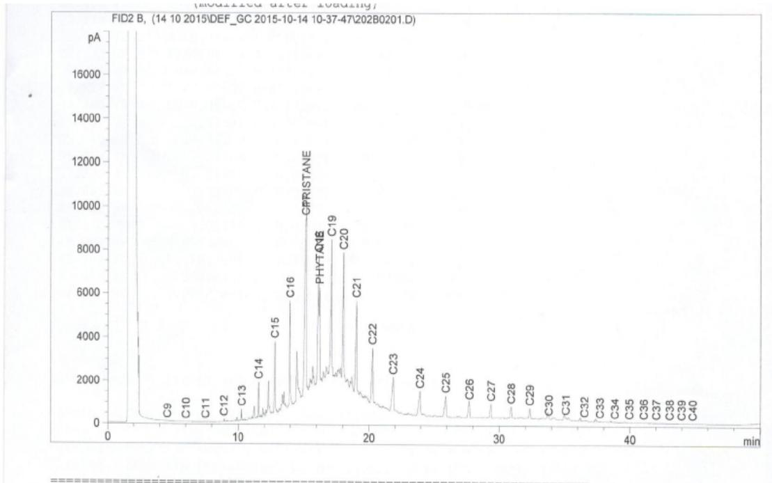
Figure 2. TPH (n-alkanes) chromatogram of oil from Ahoada soil sample
