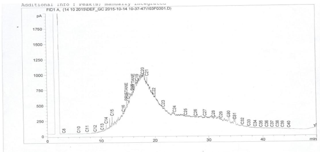
Figure 5. TPH (n-alkanes) chromatogram of oil from Bille soil sample
