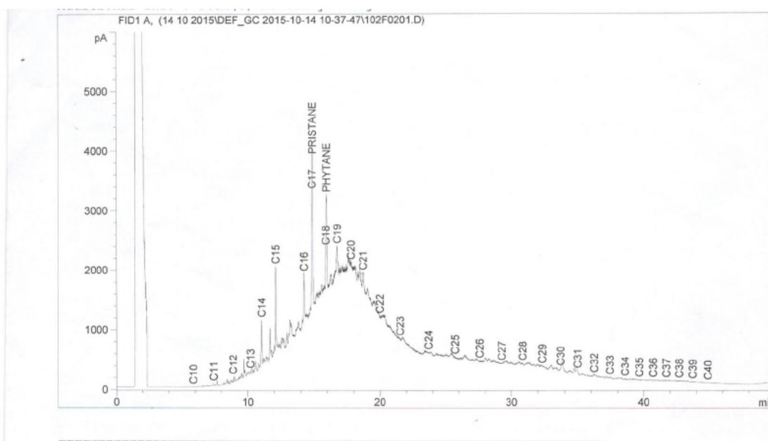
Figure 1. TPH (n-alkanes) chromatogram of oil from Etche soil sample
