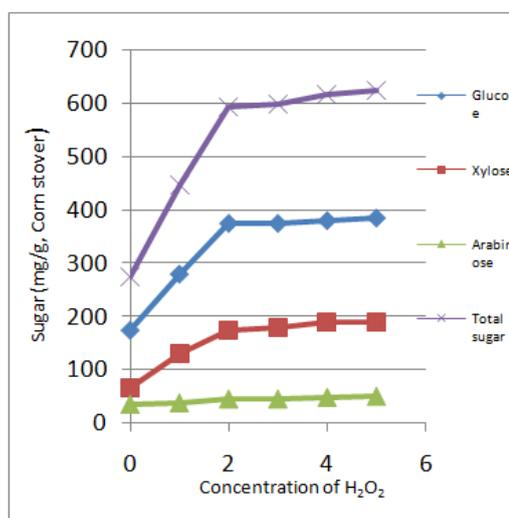
**Figure 2.** Effect of H<sub>2</sub>O<sub>2</sub> level (0-5%, v/v) for the pretreatment (pH 11.5, 35°C, 24 h) of corn stover (12.5%, w/v) on its enzymatic saccharification (37°C, pH 4.5, 120 h). The data presented are averages of two separate experiments
