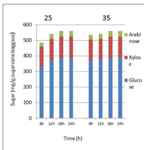
**Figure 5.** Effect of duration of alkaline  $H_2O_2$  pretreatment (2.0%, v/v; pH 11.5) of sugarcane baggase (12.5%, w/v) at two temperatures (25 and 35 °C) on its enzymatic saccharification (37 °C, pH 4.5, 6-24 h). The data presented are averages of two separate experiments
