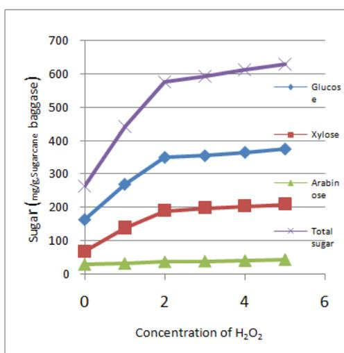
**Figure 3.** Effect of  $H_2O_2$  level (0-5%, v/v) for the pretreatment (pH 11.5, 35 °C, 24 h) of sugarcane baggase (12.5%, w/v) on its enzymatic saccharification (37 °C, pH 4.5, 120 h). The data presented are averages of two separate experiments
