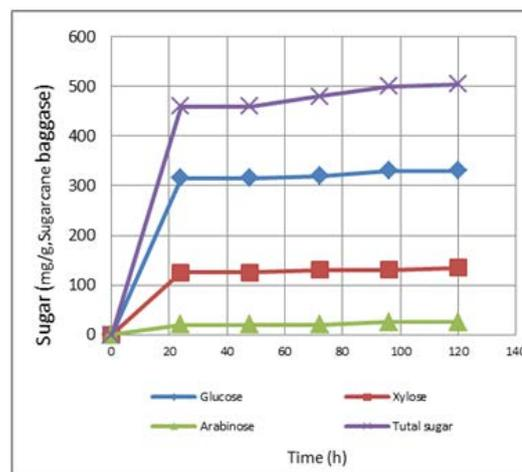
**Figure 7.** Time course of enzymatic hydrolysis (37°C, pH 4.5) of alkaline  $H_2O_2$  pretreated (pH 11.5, 35°C, 120 h) sugarcane baggase (12.5%, w/v) using *Saccharomyces cerevisiae* enzyme. The data presented are averages of two separate experiments
