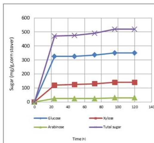
**Figure 6.** Time course of enzymatic hydrolysis (37°C, pH 4.5) of alkaline  $H_2O_2$  pretreated (pH 11.5, 35°C, 120 h) corn stover (12.5%, w/v) using *Saccharomyces cerevisiae* enzyme. The data presented are averages of two separate experiments
