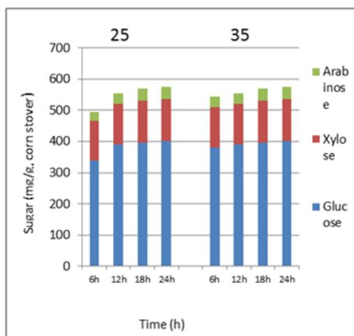
**Figure 4.** Effect of duration of alkaline  $H_2O_2$  pretreatment (2.0%, v/v; pH 11.5) of corn stover (12.5%, w/v) at two temperatures (25 and 35 °C) on its enzymatic saccharification (37 °C, pH 4.5, 6-24 h). The data presented are averages of two separate experiments
