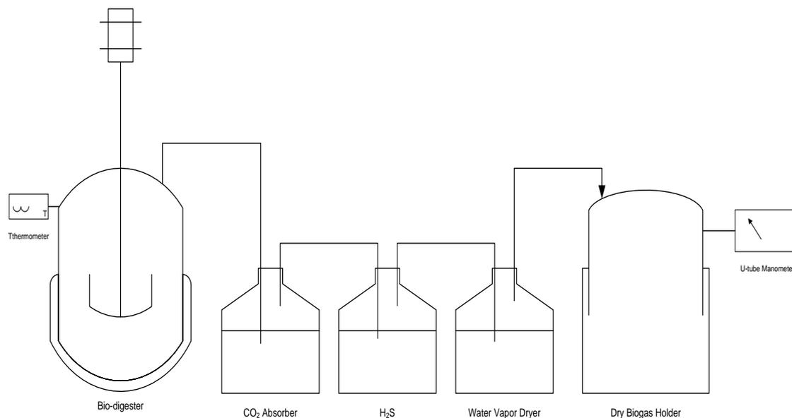
Figure 1. Flow diagram of the biogas production unit
