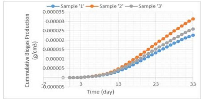
**Figure 3.** Commutative rate of biogas produced over the period of study
