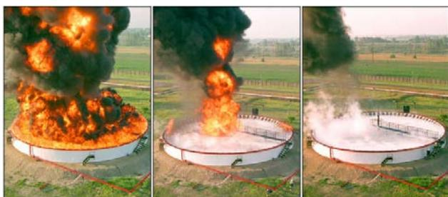
Figure 4. Fighting oil tank fire with Fixed Firefighting Foam System
