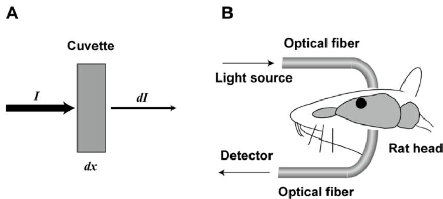
Figure 2. Block diagram of absorbance measurement. See text. A: Light intensity through the pigment solution in a cuvette,  $I$ , decreases with the thickness  $dx$  in Lambert law. B: Concentration changes in hemoglobin of rat brain were measured through optical fibers. As a light source, a halogen lamp of continuous illumination or a picosecond pulsed laser was used
