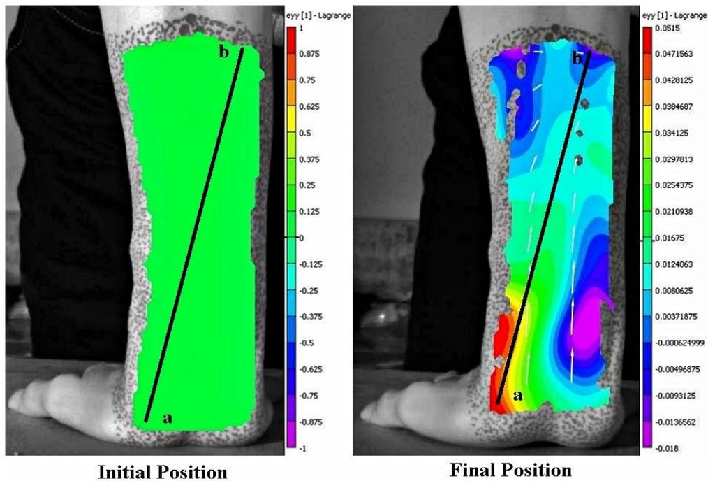
Figure 12 Strain distribution in the Y direction at Initial and final position during Wrist extension
