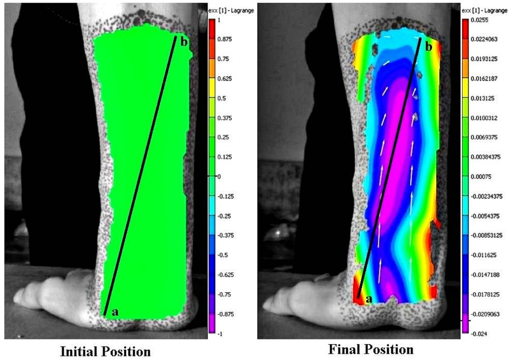
Figure 11. Strain distribution in the X direction at Initial and final position during Wrist extension
