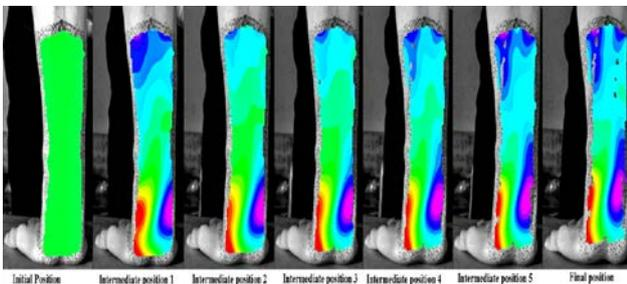
Figure 8. 2D strain distribution at different positions during wrist extension
