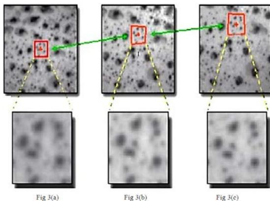
**Figure 3.** An illustration of DIC showing how the subset changes with deformation with a zooming of the image in the subset
