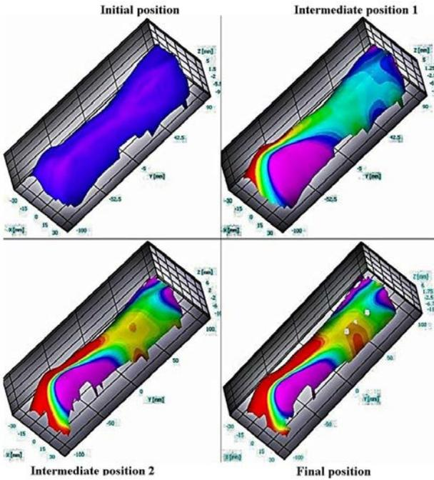
Figure 7. 3D strain distribution at different positions during Wrist extension
