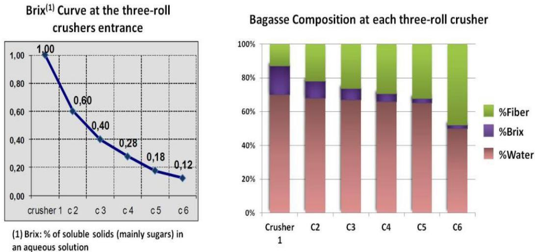
Figure 2. Typical extraction parameters in mill tandems (Source: [34])
