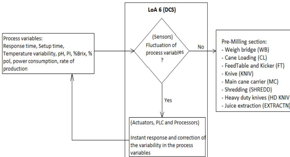
Figure 5. Experimental setup for Level 6 of automation (LoA 6) using DCS
