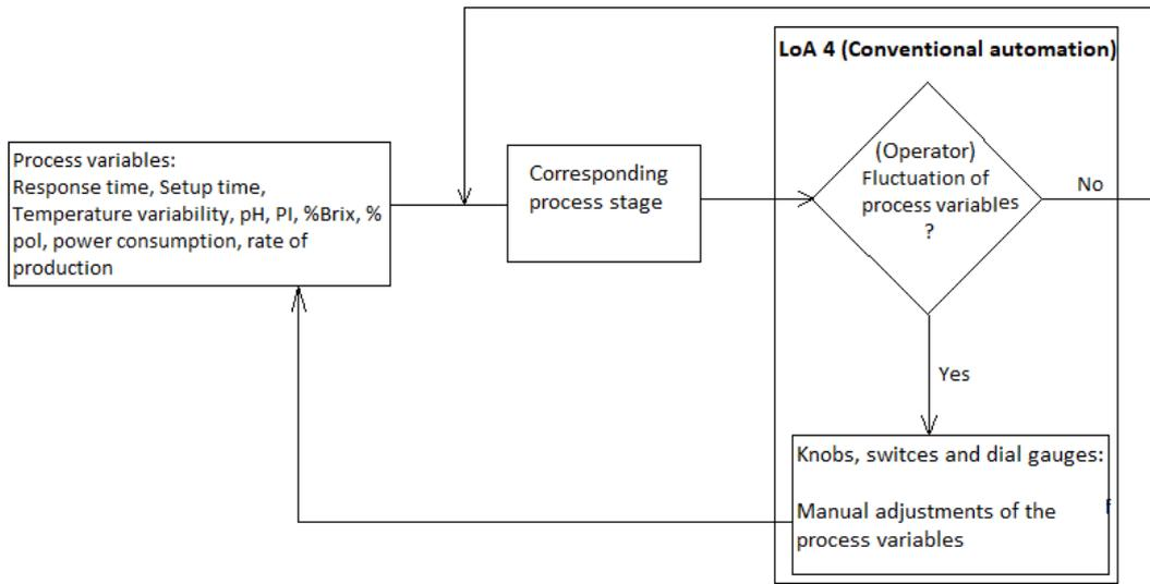
Figure 3. Experimental setup for Level 4 of automation (LoA 4) using control circuits
