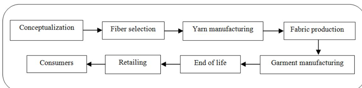
Figure 1. Sequence of the garment manufacturing process
