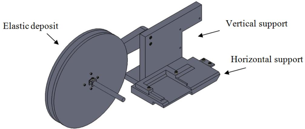
Figure 3. Design of the vertical base part of the automation system
