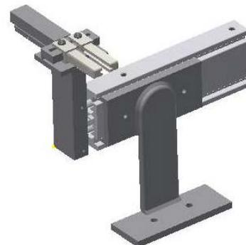
Figure 8. Rotating base that moves the slide towards the rotating module
