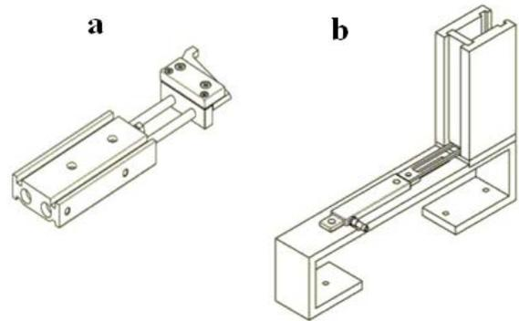
Figure 7. Cutter design and container assembly with slide: a) cutter and b) container with slide
