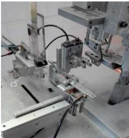
Figure 11. Complete system implemented for tie rod cutting
