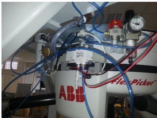
Figure 6. External vacuum connection
