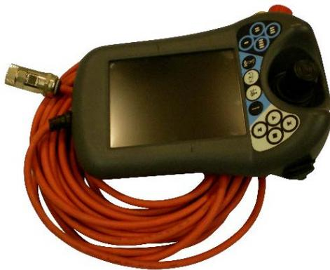
Figure 4. Pendant for ABB IRC5 [1]
