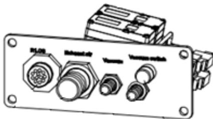
Figure 5. Panel for connections compressed air [1]
