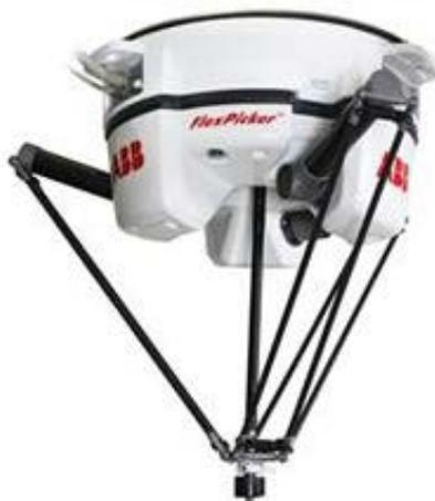
Figure 1. Robot ABB IRB 360 FlexPicker [1]
