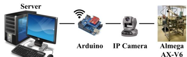
Figure 6. The architecture of client – server laboratory
