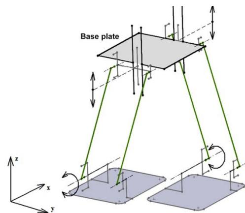
Figure 7. Kinematic arrangement of legged robot
