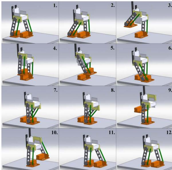
Figure 8. Walking simulation with CAD model of kinematic arrangement – variant C
