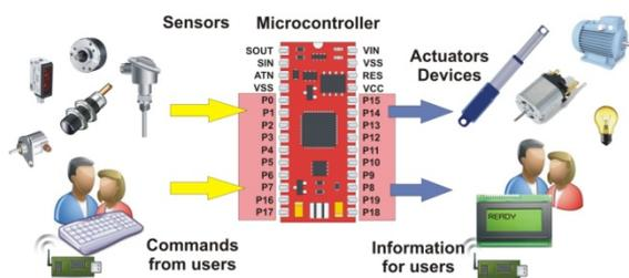
**Figure 2.** Embedded system with sensors and actuators and input or output human-machine devices
