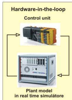
Figure 5. Hardware-in-the-loop – HIL testing and simulations
