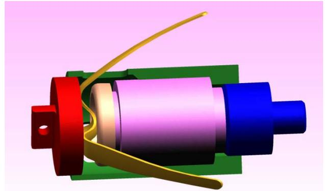
Figure 5. Concept of module with regulated bristles
