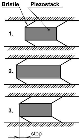
Figure 2. Piezostack vibration - Robot locomotion principle
