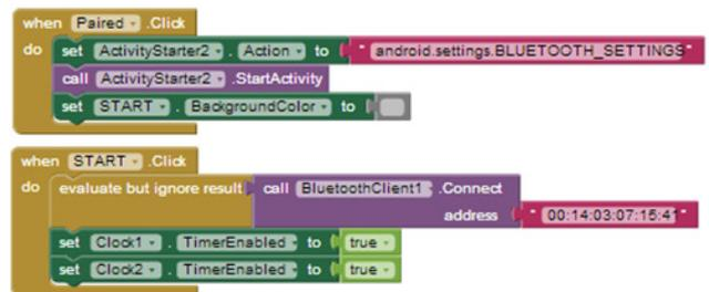
Figure 6. Block schemes for buttons for Paired and START.
