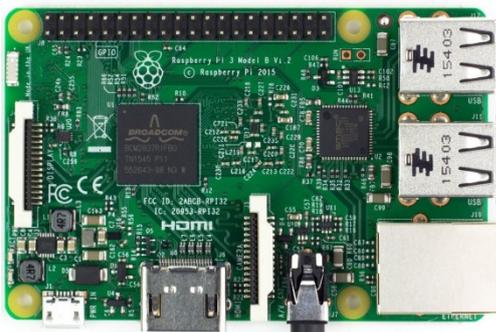
Figure 5. Raspberry pi 3 Model B single-board computer [6]
