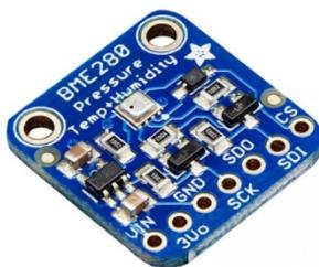
Figure 10. Pressure, temp and humidity sensor with SPI interface [12]
