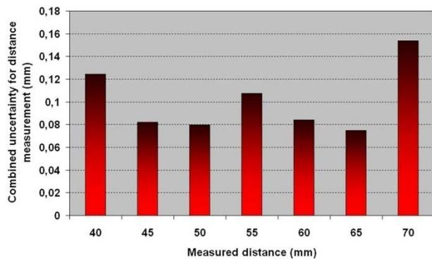
**Figure 11.** Combined uncertainty of distance measurement for optical triangulation distance sensor measured on white paper reflection surface
