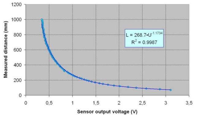
Figure 9. Calibration characteristic of optical triangulation distance sensor measured on white paper reflection surface
