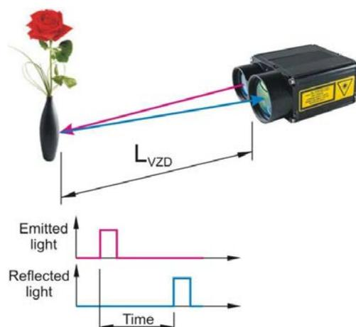
Figure 1. Time of flight position sensor principle
