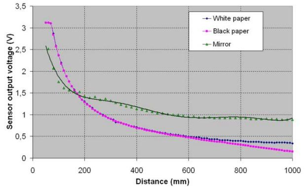
Figure 8. Static characteristic of optical triangulation distance sensor
