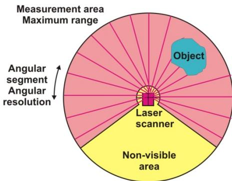
Figure 3. Time of flight laser scanner principle
