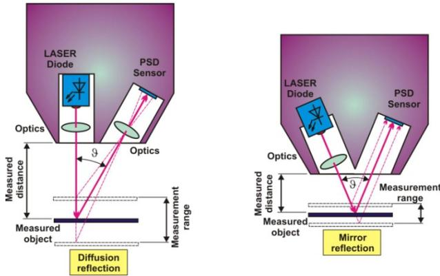
Figure 6. Optical triangulation position sensor principle
