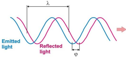
Figure 2. Phase shift between emitted and reflected light
