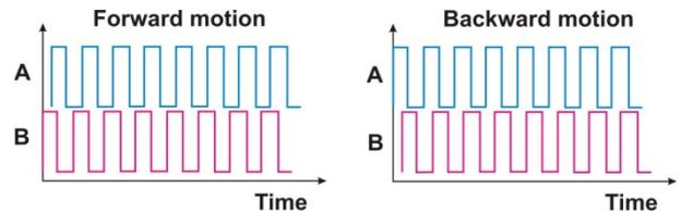
Figure 5. Recognition of motion direction of optical incremental encoder
