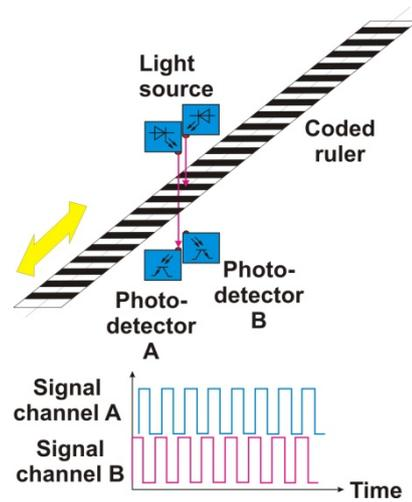
Figure 4. Incremental optical encoder principle
