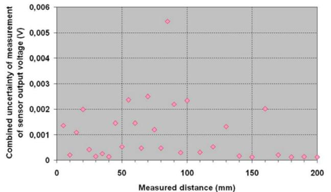
Figure 10. Combined uncertainty of measurement of sensor output voltage for optical triangulation distance sensor measured on white paper reflection surface
