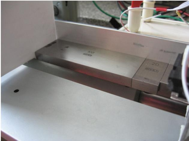
Figure 7. Experimental verification of optical triangulation distance sensor
