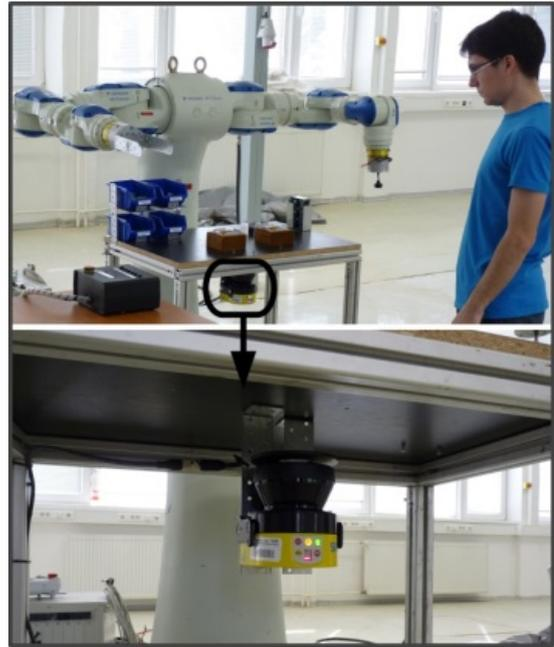
**Figure 2.** Specific robotized workplace and 2D laser scanner
