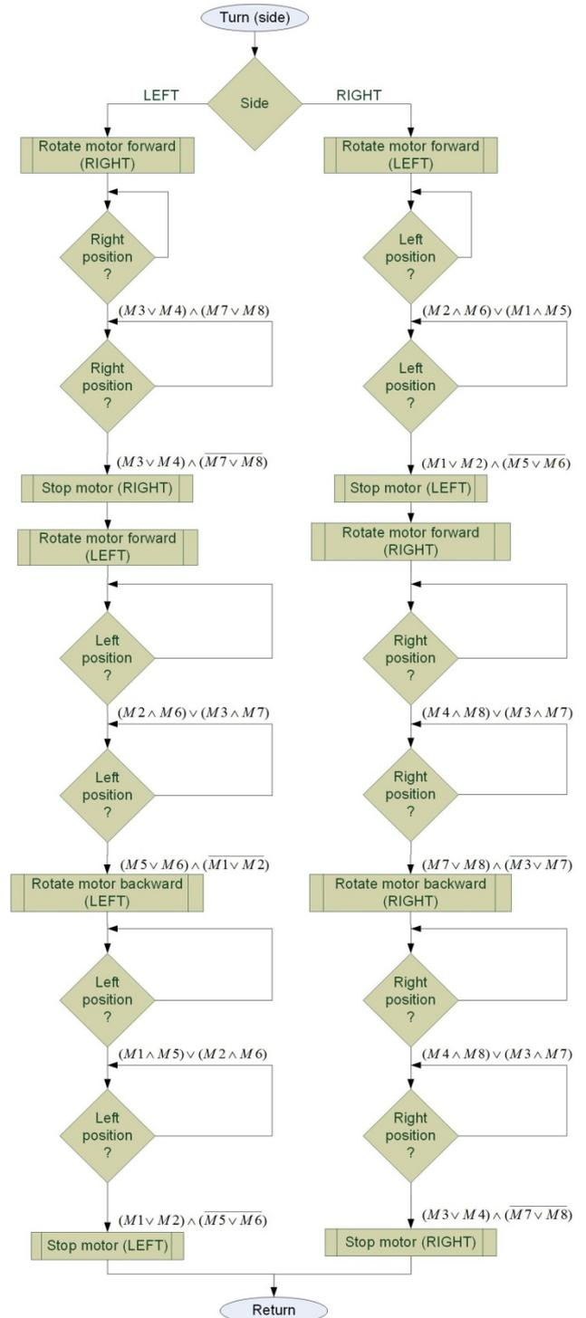
Figure 10. Algorithm for function Turning
