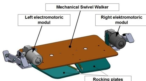
Figure 1. Design of swivel walker with electromotoric modules
