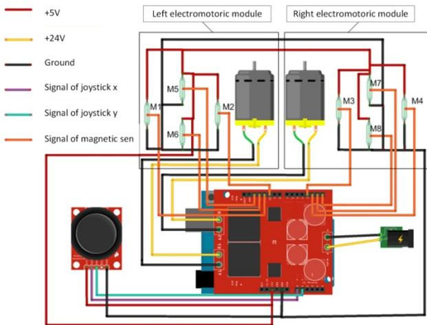
Figure 4. Connection diagram
