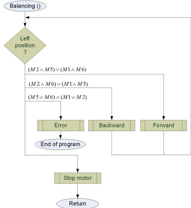
Figure 8. Algorithm for balancing left position
