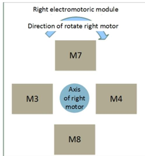
Figure 5. Placement of magnetic sensors
