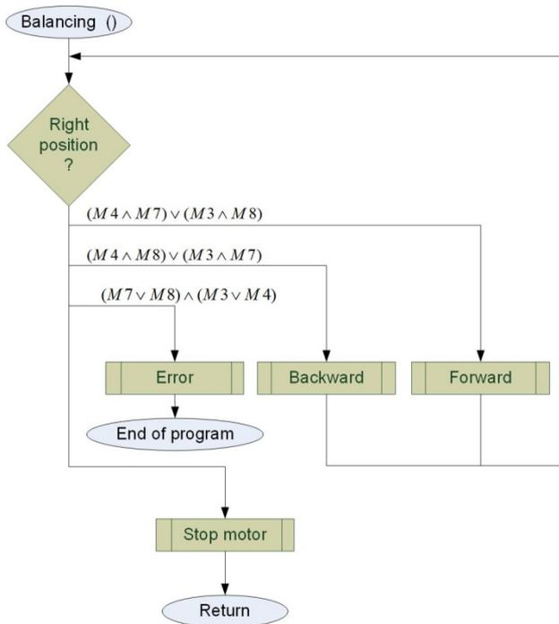
Figure 7. Algorithm for balancing right position
