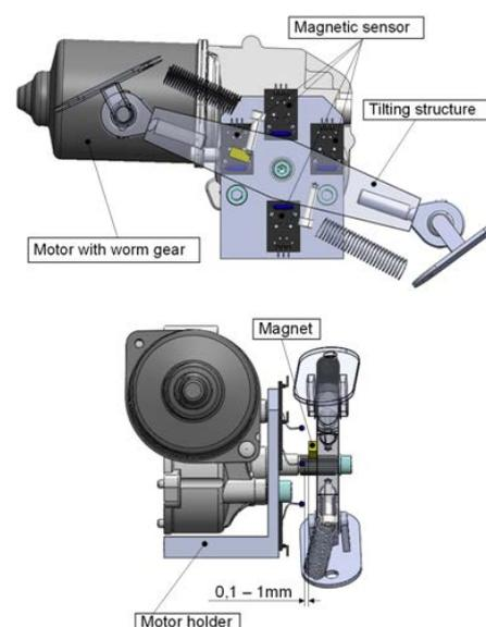
Figure 2. Proposal of magnetic sensors and magnets
