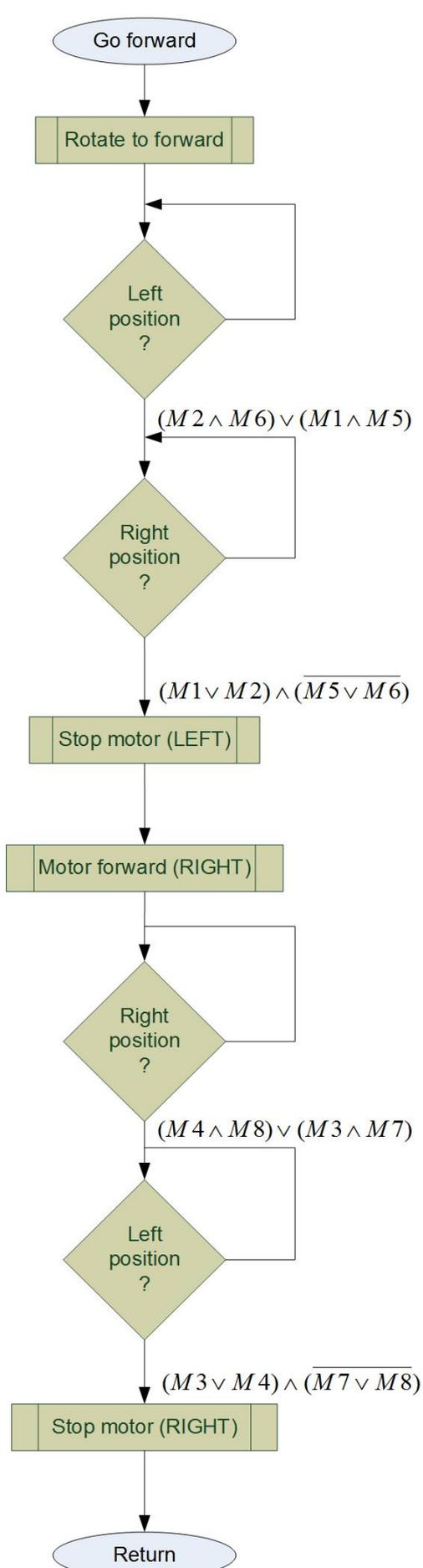
Figure 9. Algorithm for function Go forward
