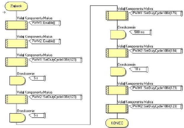
Figure 12. Control algorithm for second test of device flying
