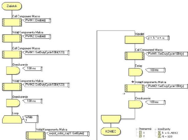
Figure 11. Control algorithm for test of device flying
