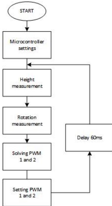
Figure 14. Algorithm of stable condition control
