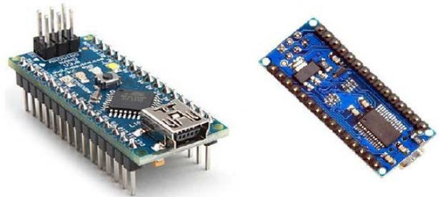
**Figure 6.** Control unit Arduino Nano
