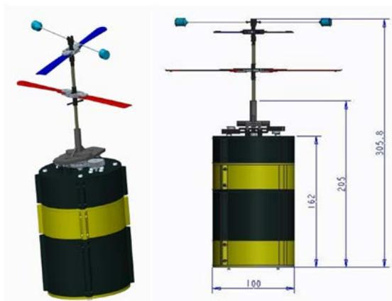
Figure 1. Coaxial-copter (Flyself) 3D and 2D model
