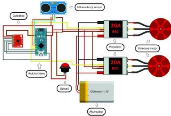
Figure 9. Wiring diagram
