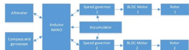
Figure 2. Basic controlling concept
