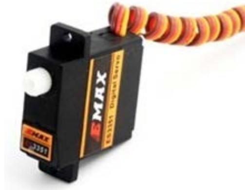
Figure 4. Servomotor Emax ES3351
