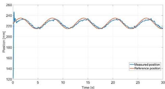
**Figure 7.** Experimentally measured position of air bellow top platform compared with reference signal
