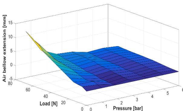
Figure 2. Measured air bellow extension with changing external load and inner pressure in the bellow
