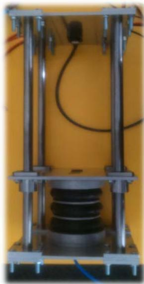
**Figure 6.** Measuring stand for air bellow with ultrasonic sensor, fixed bottom platform, moving top platform
