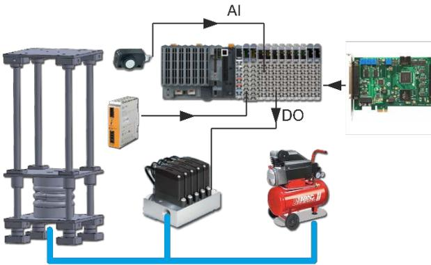
Figure 4. Hardware of control system
