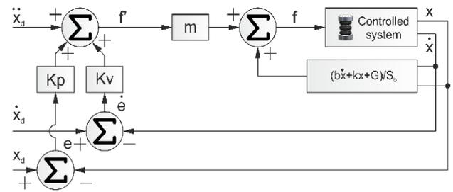
Figure 5. Control system of trajectory tracking
