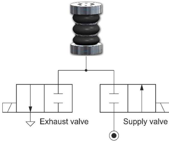
Figure 3. Control of pressure in air bellow by two 2/2 NC valves
