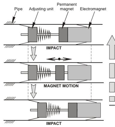
Figure 8. Simplified motion cycle of in-pipe machine based on inertial stepping principle
