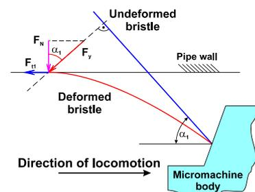
**Figure 4.** Forces on bristle tip in forward locomotion
