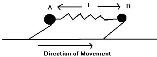
**Figure 2.** Worm-like in-pipe locomotion principle – directional friction principle
