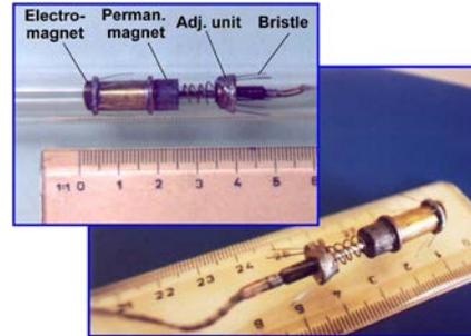
Figure 7. In-pipe machine based on inertial stepping principle
