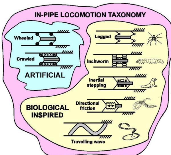
Figure 1. Ways of in-pipe machine locomotion
