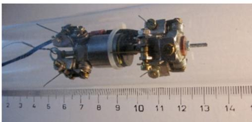
**Figure 3.** Worm-like in-pipe machine based on directional friction principle. 1 – piezoactuator, linear motor; 2 – head bristle plate; 3 – back bristle plate; 4 – bristles; 5 – screw; 6 – pipe
