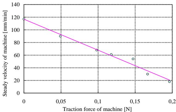
Figure 6. Machine velocity versus traction force of machine
