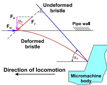
Figure 5. Forces on bristle tip in backward locomotion
