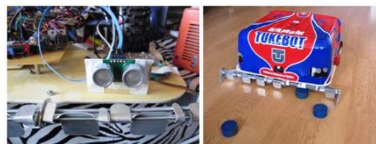
Figure 3. Ultrasonic sensor on for mobile robot navigation
