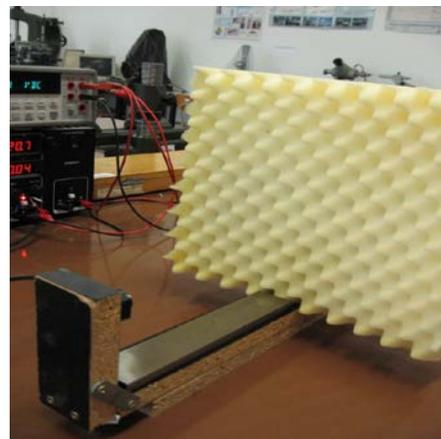
**Figure 7.** Testing of ultrasonic sensor with compliant obstacle
