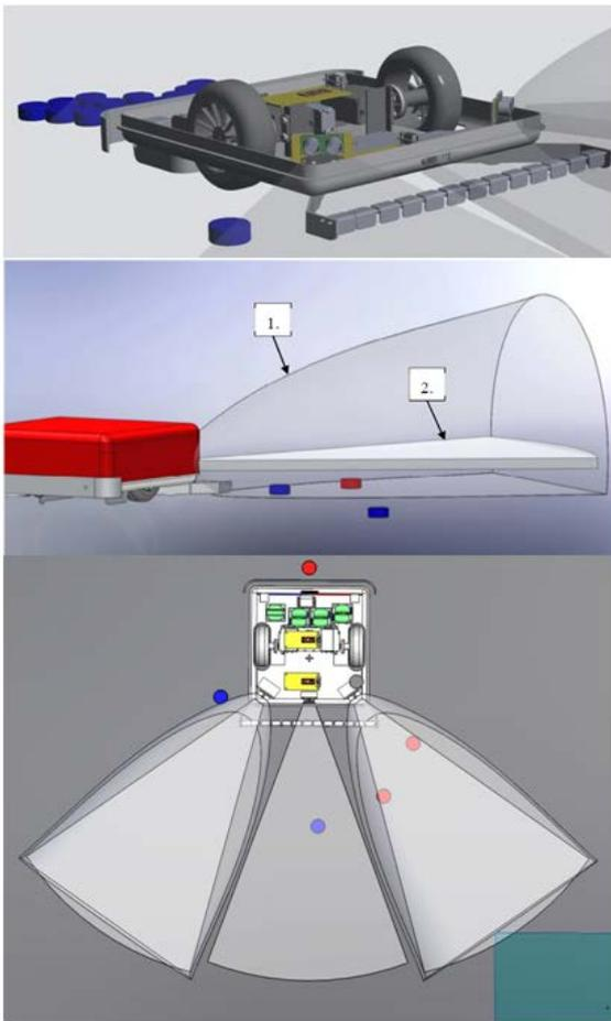
**Figure 4.** Sensor for puck collecting robot (1 – ultrasonic sensor active field), (2 – infrared sensor active field)
