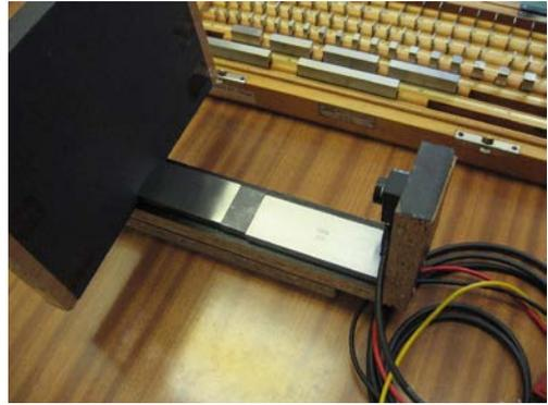
**Figure 5.** Testing of ultrasonic distance sensor
