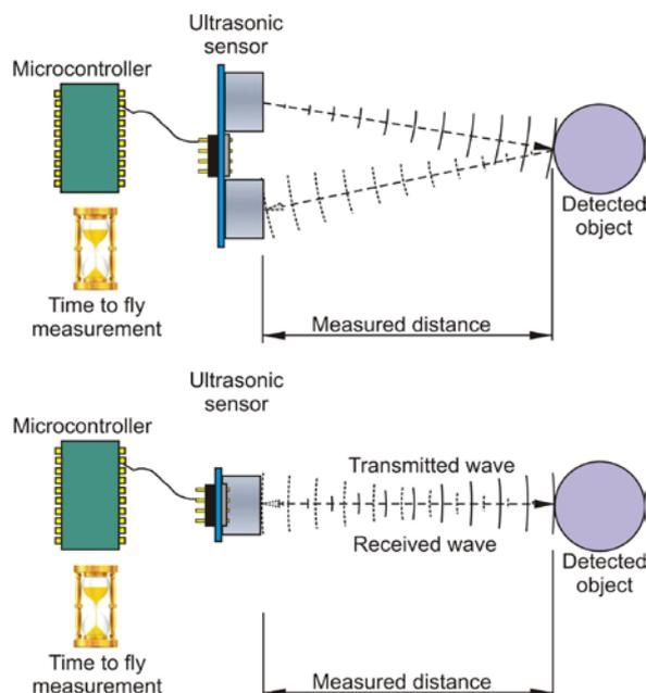
Figure 1. Ultrasonic sensor working principle
