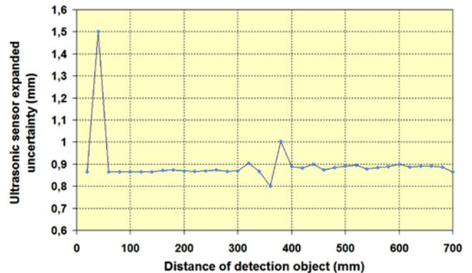
**Figure 10.** Standard uncertainty of measurement for measurement chain with ultrasonic distance sensor
