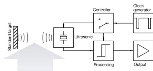
Figure 2. Ultrasonic sensor block scheme [4]
