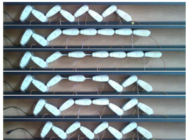
Figure 11. Experiment with snake robot LocoSnake
