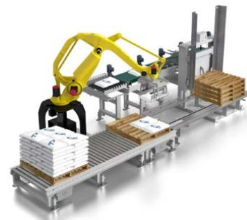
Figure 2. Configuration of industrial robot for palletizing of heavy objects to transport pallet
