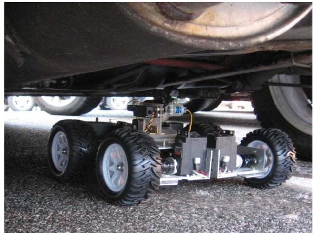
Figure 1. Mobile robot with divided chassis
