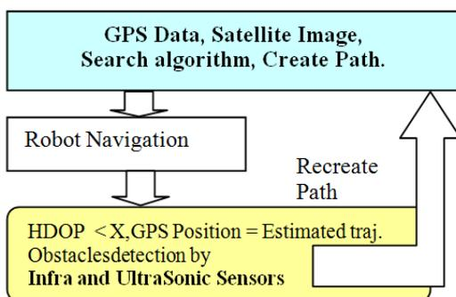
Figure 10. Extended navigation algorithm with sensors
