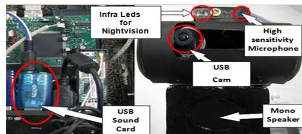
Figure 12. Audio and video system, motion detection
