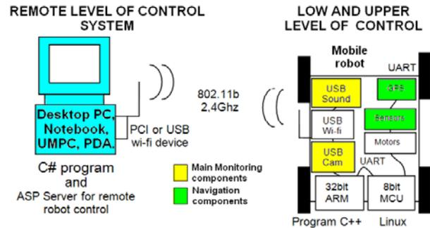
Figure 3. Principle scheme of mobile robot control based on GPS navigation
