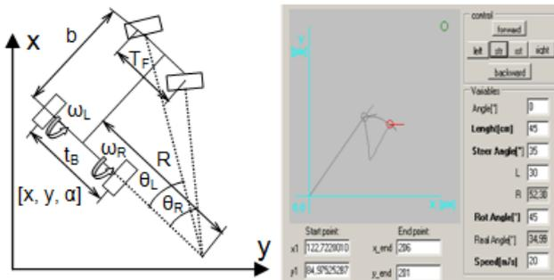
Figure 2. Kinematics scheme for estimation of position in 2D
