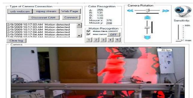
Figure 13. Video system for motion detection
