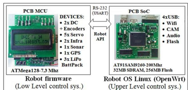
Figure 4. Principle scheme of control system of mobile robot
