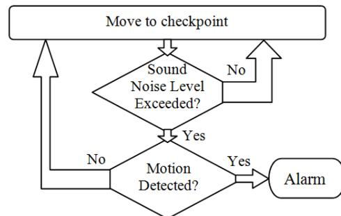
Figure 11. Audio and video system alarm principle
