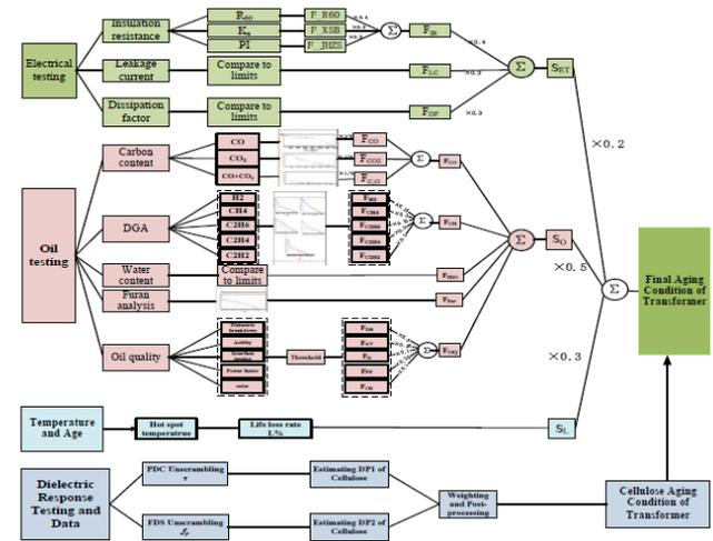
Figure 2. Flowchart for assessment of transformer aging with multi parameters [1]
