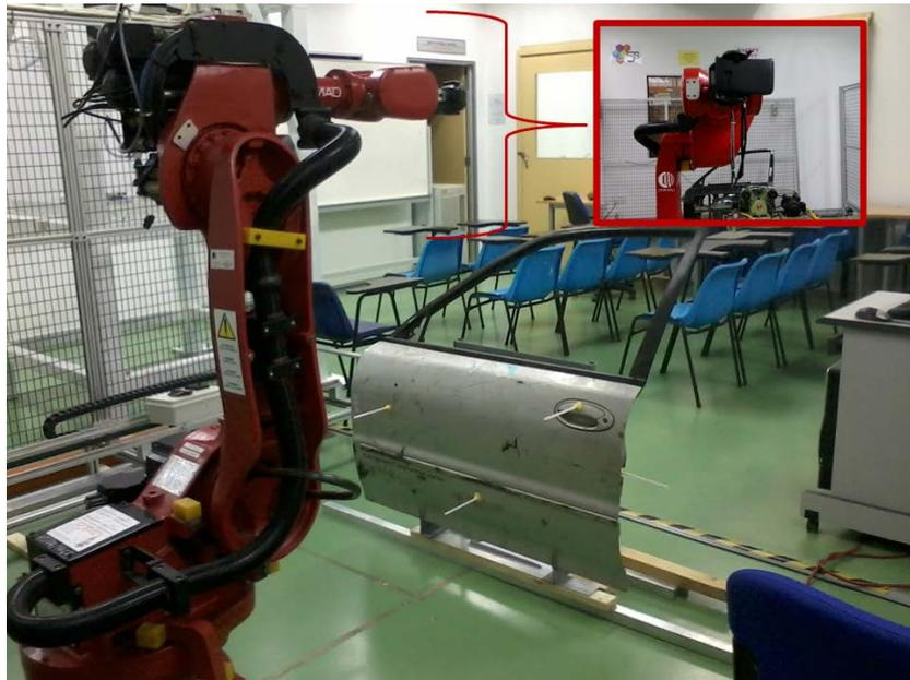
**Figure 1.** The car door (works piece) is shown stood up, and the end effector has a camera installed. The front view of the end effector is marked in the box within the figure
