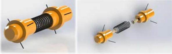
Figure 2. CAD model of in-pipe robot
