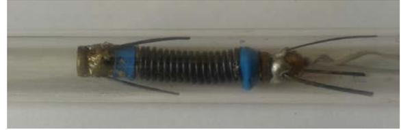
Figure 8. In-pipe robot in the pipe
