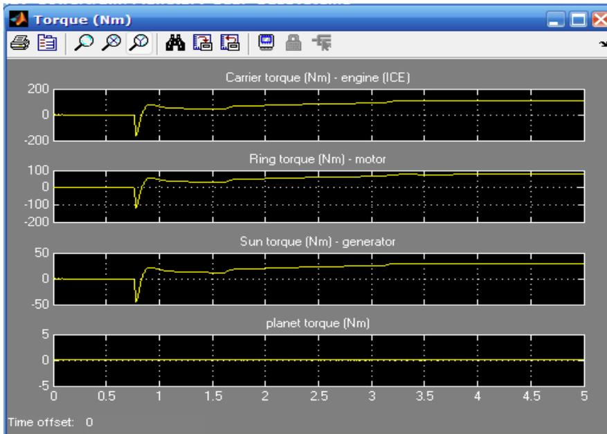
Figure 16. Planetary Gear torque, power Subsystem result
