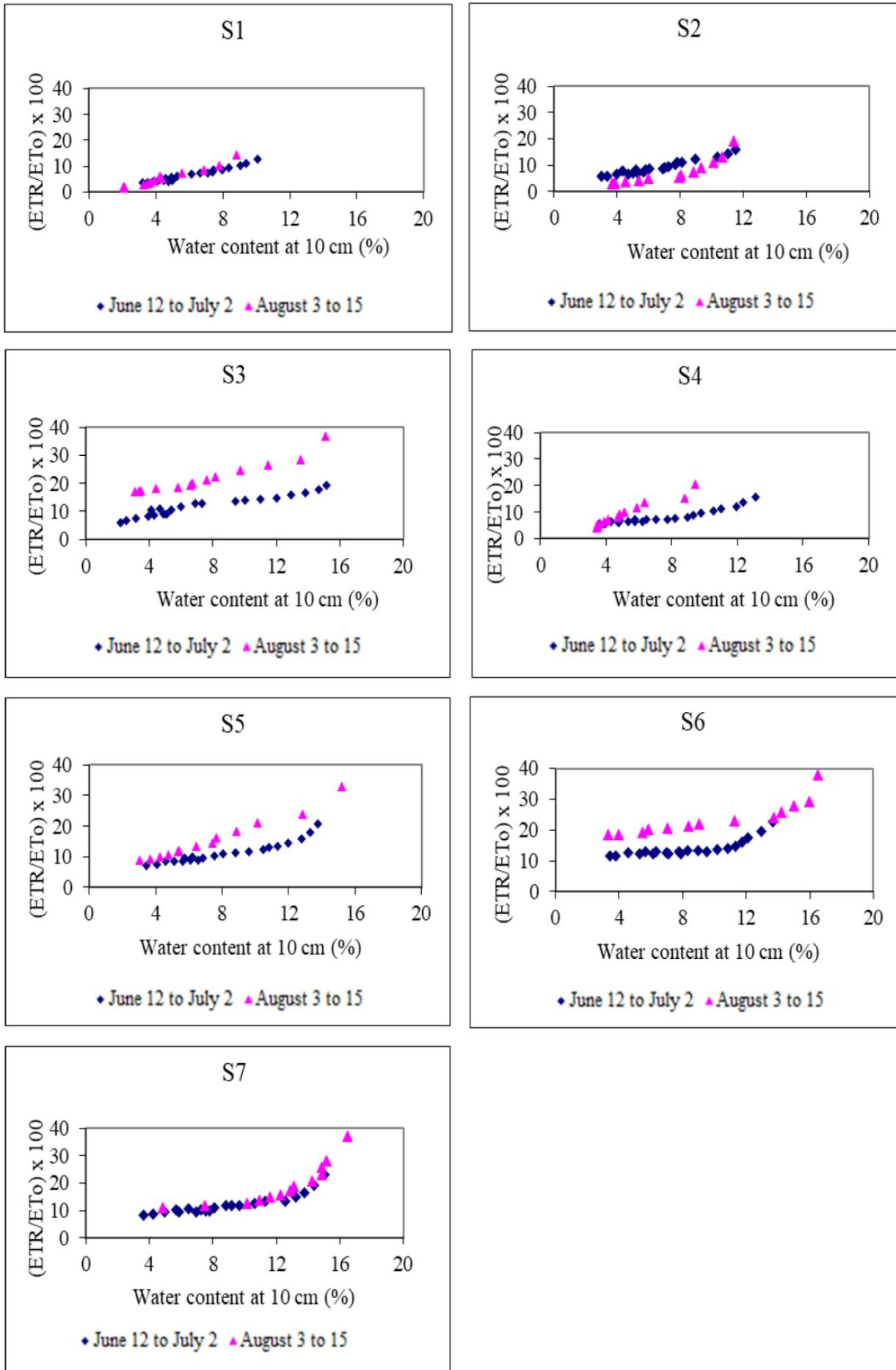
Figure 6. Evolution of the ETR/ETo ratio as a function of water content at 10 cm depth for two dry periods
