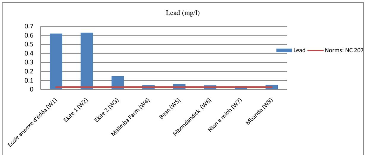
Figure 6. Concentration of Lead in the various of sampling borehole
