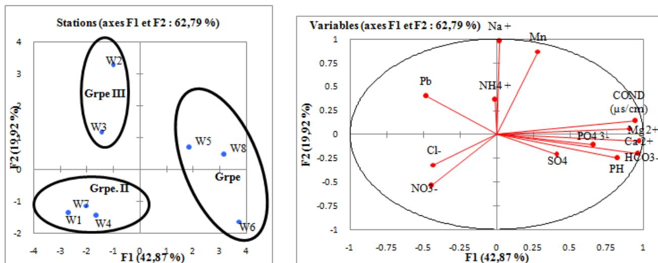
Figure 9. PCA on distribution of the physicochemical parameters in the 8 well
