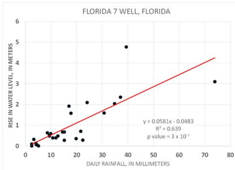
**Figure 4.** Rise in water level versus rainfall at the Florida 7 well, Florida. Data courtesy of USGS
