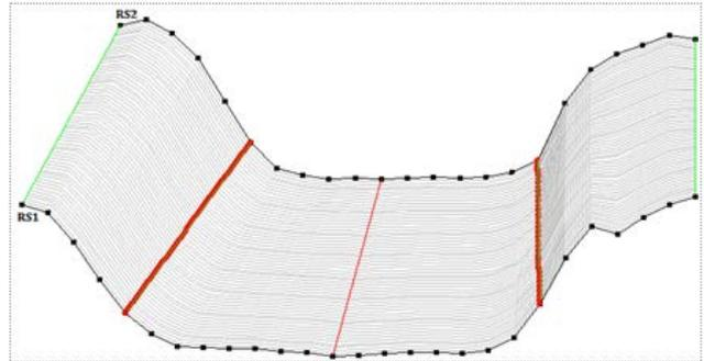
Figure 3.c. Interpolated cross-sections plots Between RS2 and RS1
