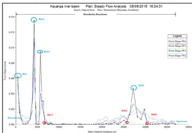
Figure 8. Friction slope distributions
