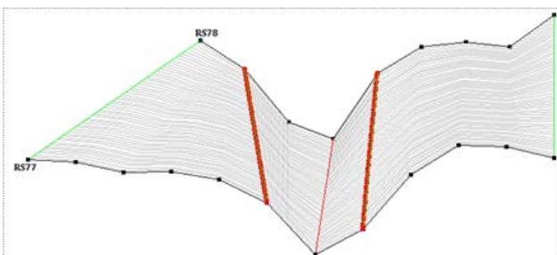
Figure 3.a. Interpolated cross-sections plots Between RS78 and RS77
